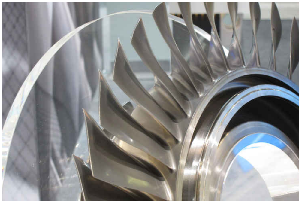
Figure 1.6: Monolithic construction. From [11].
